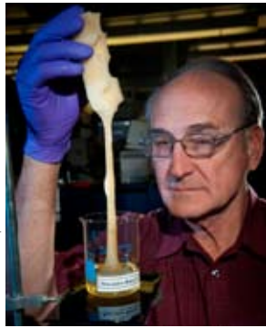
Ron Simandl, one of the RonJohn inventors, degrades polyurethane foam by dipping it in RonJohn .
